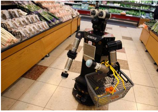
Fig 3.1 The automatic follow-me shopping cart example (Robot in image: Robovie-II)
