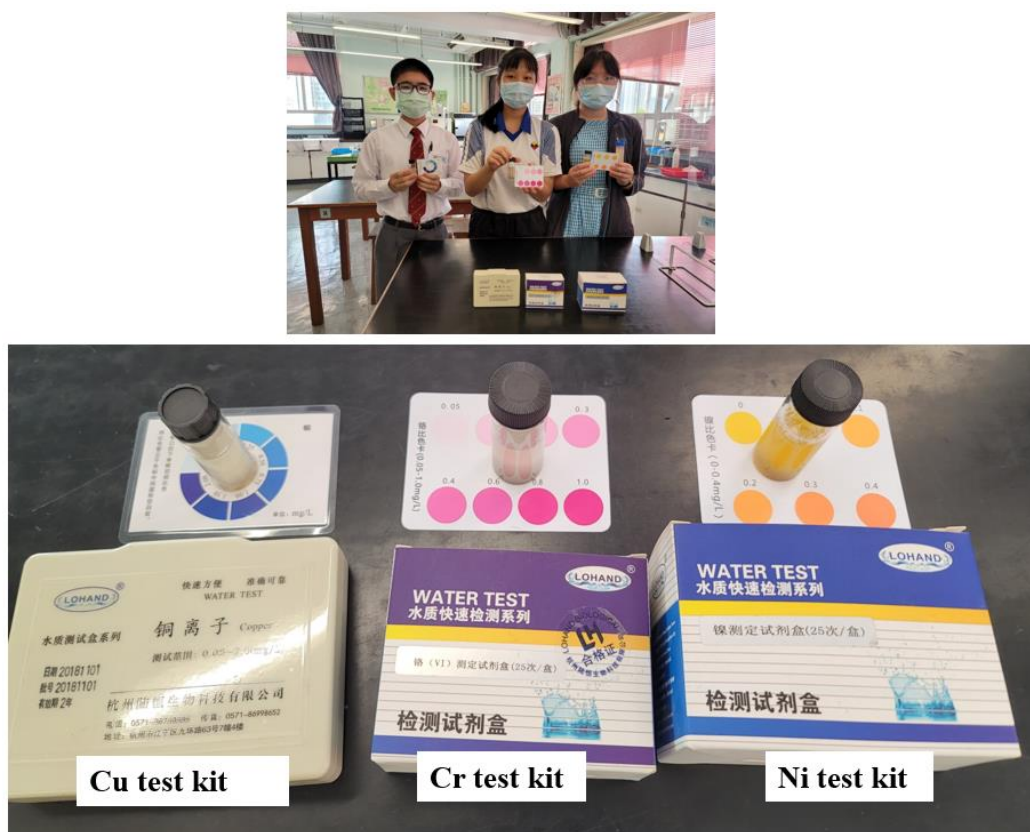
Fig. 13 Test for some heavy metals in the sediment extract using commercial test kits, which showed undetectable level of Cu, Cr and Ni
