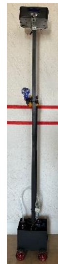
Figure 5. Final version of the prototype: Susanito, an autonomous robot measuring body temperature: support to reduce infections in lines. Own photography.
