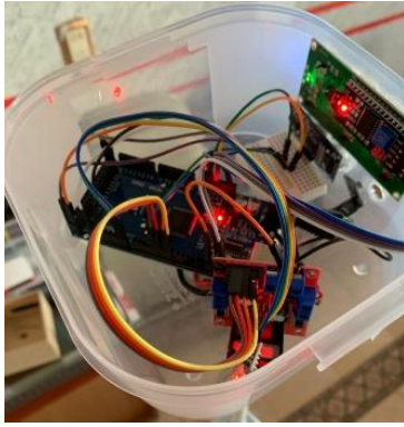
Figure 2. Internal view of the temperature sensors and display. Own photography.
