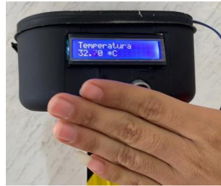
Figure A.6. Temperature sensor and display communication test. Own photography.
