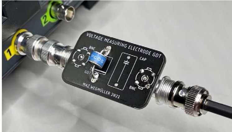
Figure 22: The small PCB is connected directly to the oscilloscope.
