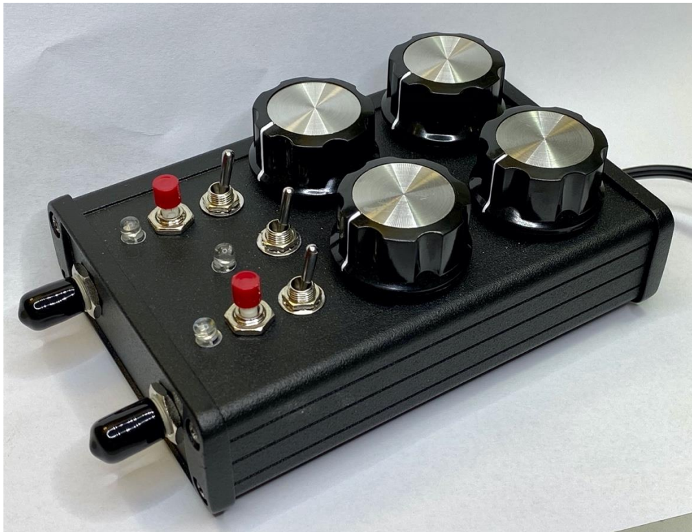
Figure 14: The ready assembled interrupter in the aluminum housing.
