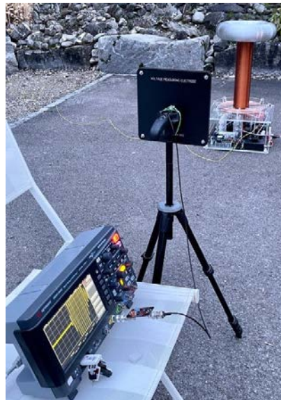
Figure 20: The experimental setup of the voltage measurement via a measuring electrode.
