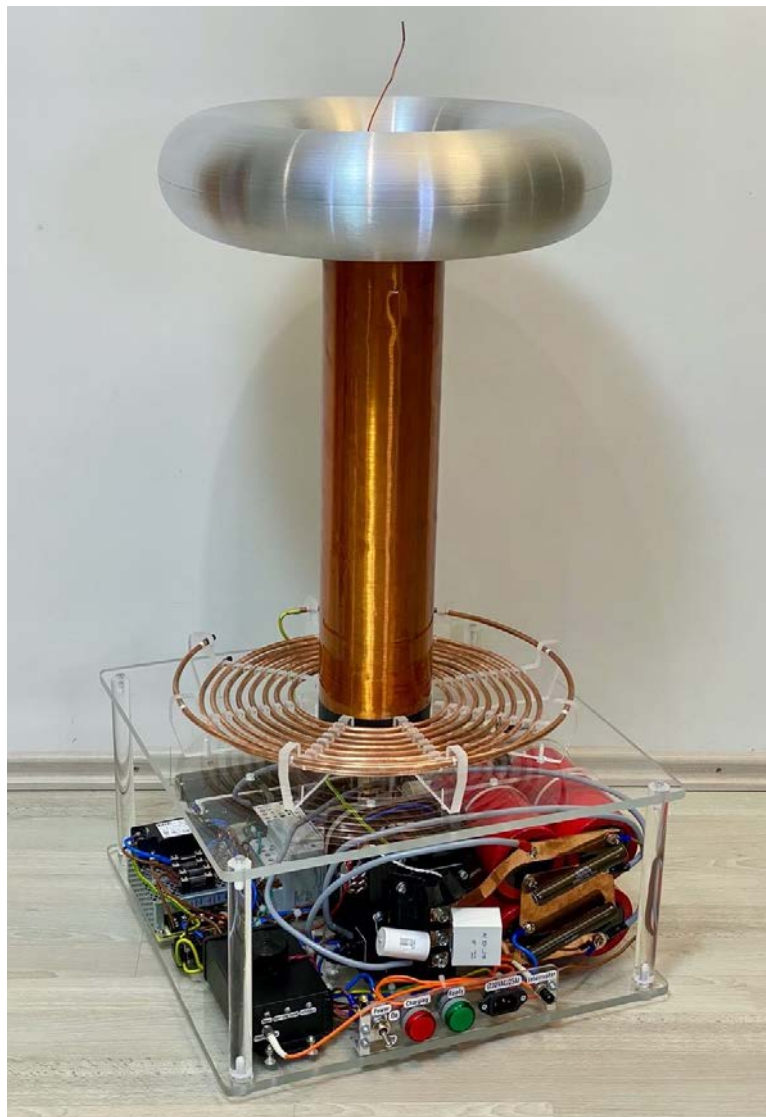
Figure 5: An audio modulated DRSSTC with medium power output.
