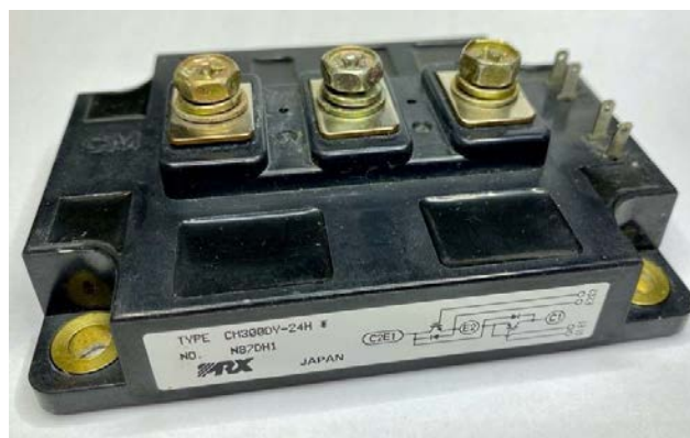
Figure 11: A CM300DY-24H IGBT half bridge module from Powerex.
