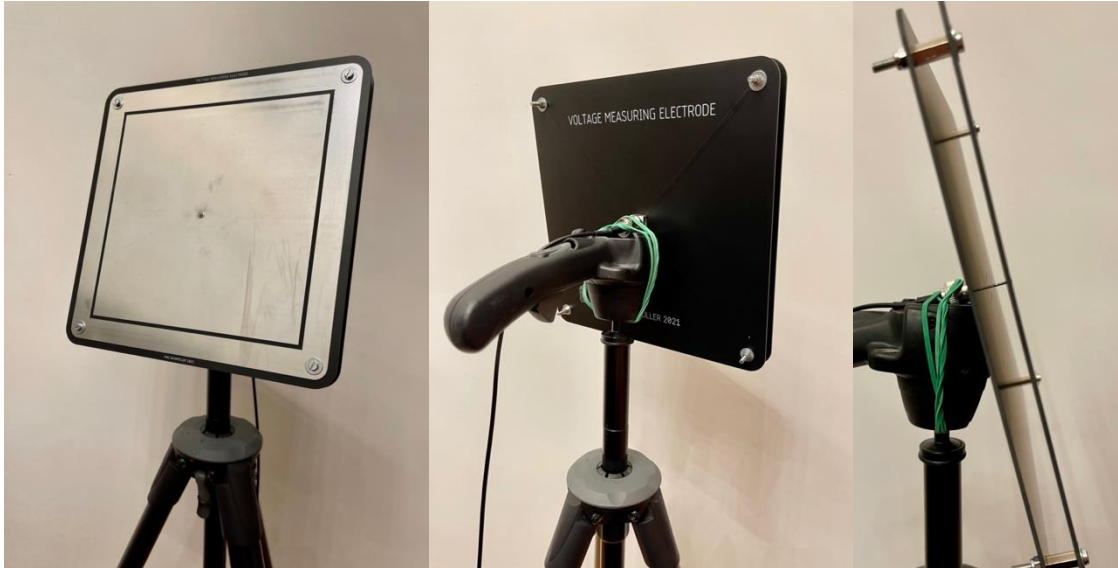
Figure 21: The assembled measuring electrode on the stand from the front, back and side (fLTR).
