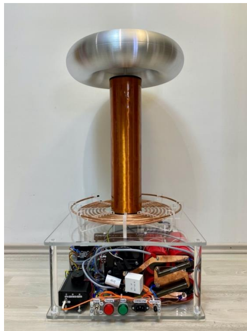
Figure 8: The DRSSTC with the eye-catching and characteristic secondary coil.
