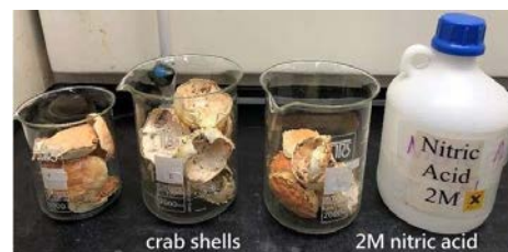
demineralization of crab shell (removal of calcium carbonate using 2M nitric acid)
