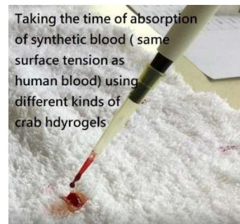
Fig 3.9 Synthetic blood, same surface tension as human blood. Fig. 3.10 Absorption of synthetic blood by crab hydrogels Time was taken for the absorption of 10 microlitre synthetic blood by different samples.
