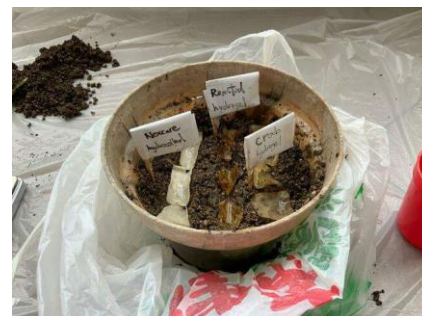
Fig. 3.14 Samples in soil for bio-degradation
