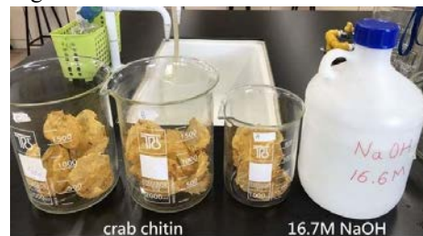
Deacetylation of chitin to chitosan using 16.7M NaOH
