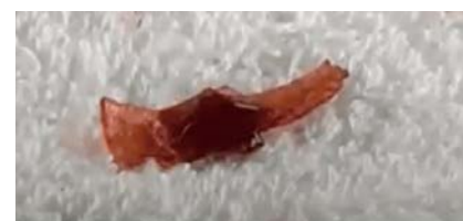
Measuring FSA Free-swell absorbency of crab hydrogel bio-dressings using synthetic blood
