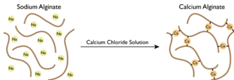
Figure 3. Gel principle of sodium alginate
