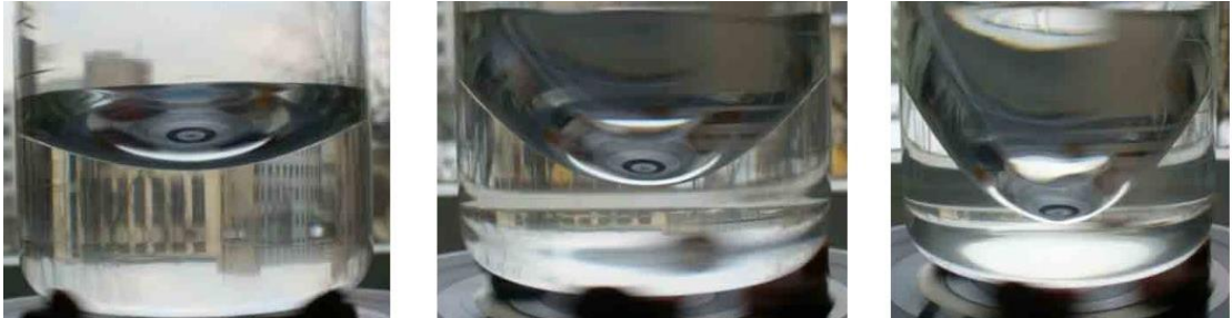
Fig. 2.7 Changing the shape of the lens depending on the speed of rotation
