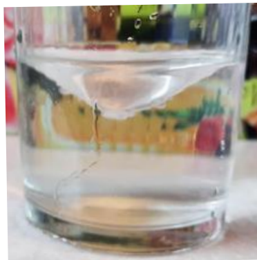
Fig. 2.6 The lens is formed by the rotation of the liquid
