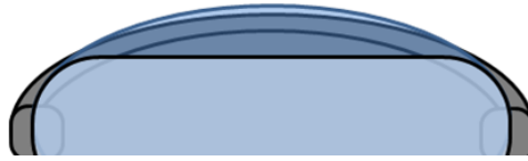
Fig. 2.3 Creating a lens using surface tension
