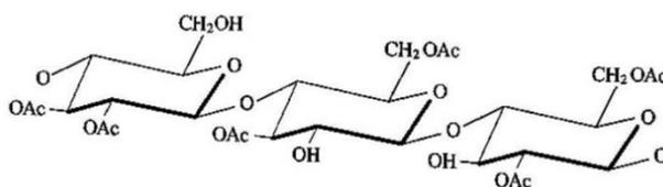
Figure3. Polymer network of cellulose diacetate [8]
