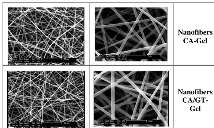
Figure4. SEM images of nanofiber scaffolds with and without extract in two magnifications
