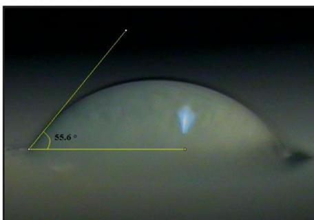
Figure5. Contact angle of water droplet with the surface of nanofiber scaffold containing extract
