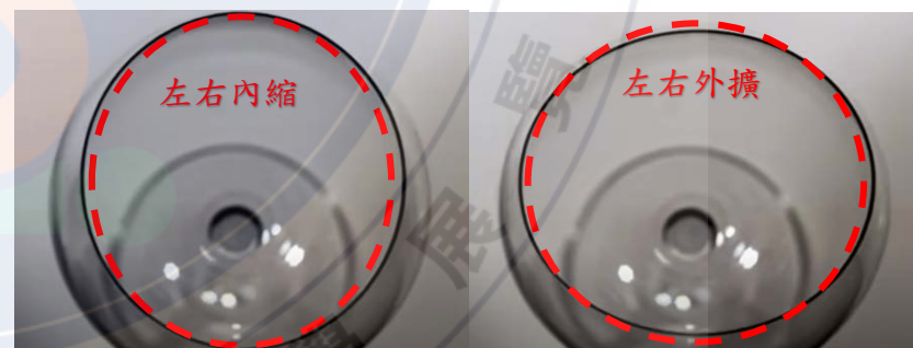
玻璃杯振動俯視圖(紅圈：未振動時原始口徑) 取自：Wine glass resonance in slow motion.
